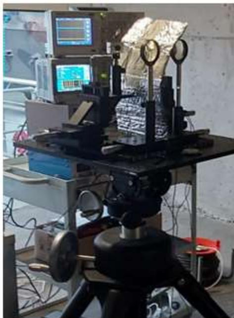
Figure 2. Experimental LRF setup on the breadboard.
